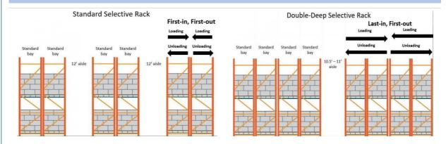
**Increase in storage capacity** compared to selective pallet racking.
